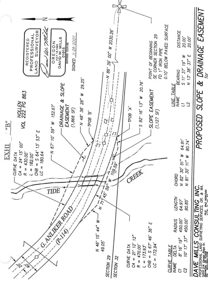
PROPOSED SLOPE & DRAINAGE EASEMENT
